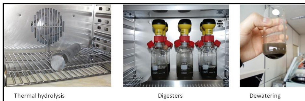
Figure 4: Laboratory tests on thermal hydrolysis, digestion and dewatering
