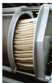
Figure 7 - Hydraulic Press System And Functional Principle Of Drainage Elements, On The Right Side A Opened Cylinder With Drainage Elements. [Boehler et al 2003].
