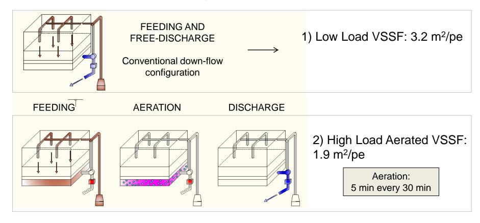
Equipment: small air blower connected to perforated pipes on the bottom of the bed
