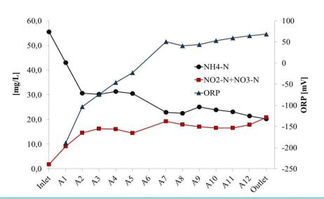
NO<sub>X</sub>-N produced +18 mgN/L TKN removed -59 mgN/L
