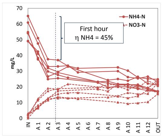
NH<sub>4</sub>-N concentration in the bed not significantly reduced by intermittent aeration on the bottom.
