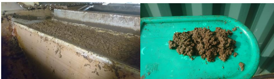
Figure 4: Sludge layer on top of the T-DAF and after sampling
