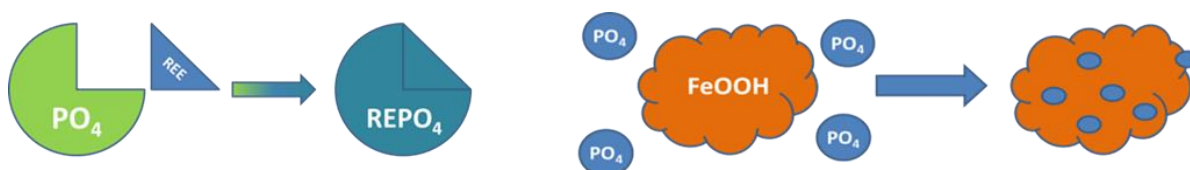
Figure 1. Depiction of phosphate removal reaction mechanism of RE vs. Fe
