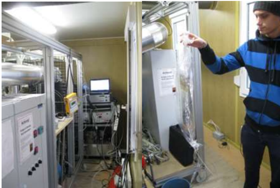
Figure 2: Testing of exhaust air from a small experimental dryer (HUBER SE 2012)
