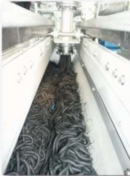
Figure 6: Extruder forming pellet strains
