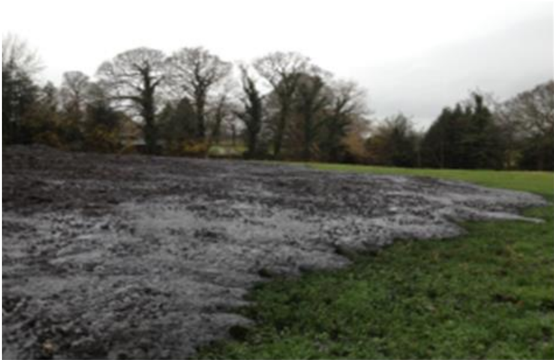
Figure 1: Collapsed Biosolids stockpile in 2012 wet weather.
