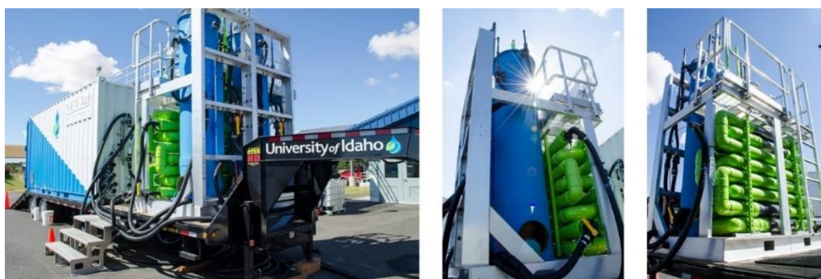
Figure 1. N-E-W Tech process mobile research trailer. Reactive filters are blue, plug flow reactors are green, and the white/blue process control container contains water pumps, reagent dosing controls, air compressor, air dryer, oxygen concentrators, ozone generator, programmable logic controller, sensors, digitally controlled valves, system controls, power-process controls, lights and heat.
