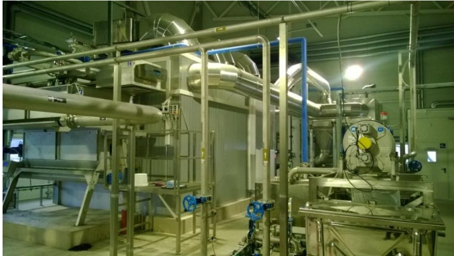
Figure 1: Modern HUBER belt dryer in Lithuania with screw press for dewatering [HUBER SE 2012-2015]
