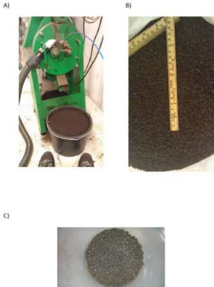
Figure 5: Photos of A) Pilot pelletizer, B) MINORGA® 10 – 1 – 5, C) MINORGA® 10 – 3 - 14 5
