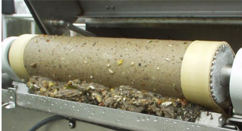
Figure 6: The solids mat discharging from a microscreen.
