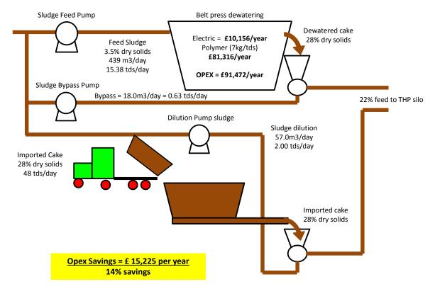
**Option 3** – would to particularly select the thickened SAS for back-mixing. There are two advantages to this: 1) that thickened SAS will be of a higher dry solids so the same volume contains more solids, and 2) SAS requires more polymer for pre-THP dewatering and achieves a lower dry solids result then primary; so removing as much SAS as possible from the pre-THP dewatering feed will mean less polymer required and higher cake dry solids.
