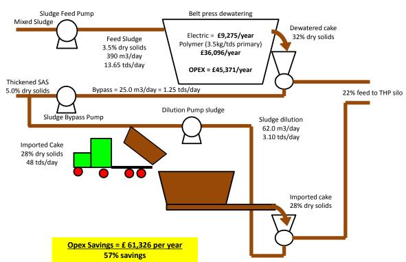
Option 3 – Bypass and Back-mixing using thickened SAS
