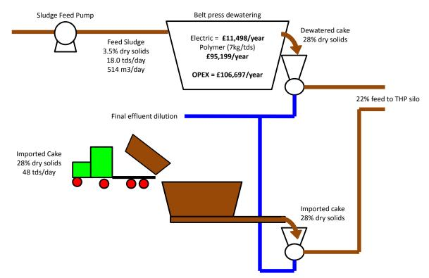
**Option 2** – is to use the feed sludge to the pre-THP dewatering – as is the case at Chertsey. The flows and Opex for this option are shown.
