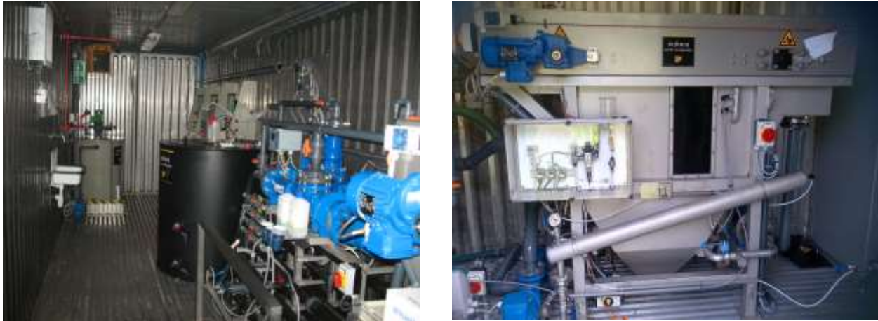
Figure 2: The pilot DAF set-up inside the 40" at OlburgenWWTP (left picture: pipe flocculator with chemical dosing, right picture: DAF pilot).
