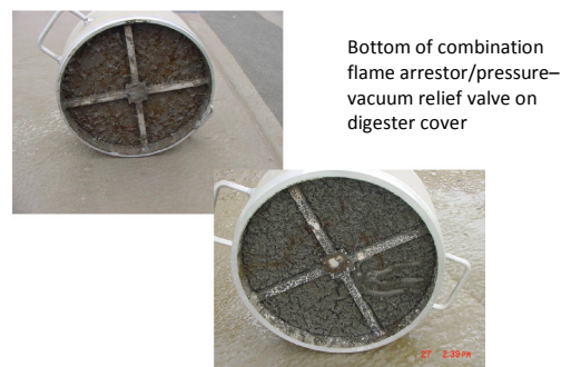
Figure 1: Impacts of AD Foaming clogged gas handling equipment
