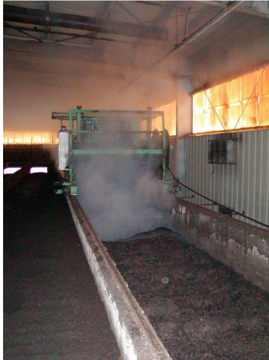
Photo 5: Moisture Released through Agitation w/Aeration: Bay 1, Merrimack Study
